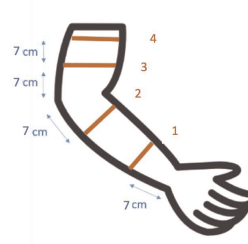
Fig. 2 Layout of lymphometer sensors
